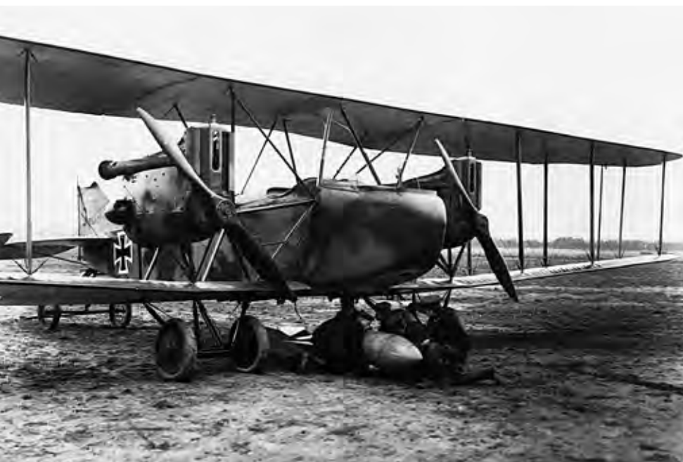
Source 5.24 German airmen attach a 100-kilogram bomb to the underside of a Gotha bomber.
